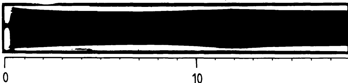
FIG. 2. 'Smooth transition' ice layer for Re_{4h} = 36000 , \theta_c = 8 and Pr = 13 .
